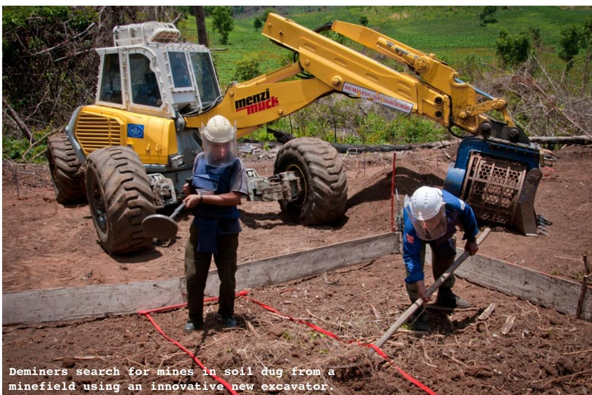
Deminers search for mines in soil dug from a minefield using an innovative new excavator.
