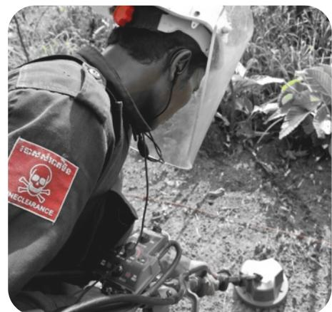
A HALO deminer uses an HSTAMIDS, a conventional metal detector which also incorporates ground-penetrating radar, to search for landmines. This kind of cutting-edge technology is one of numerous ways HALO is improving cost-effectiveness and speeding up its life saving work. The more efficient that we can make mineclearance, the more value-for-money we provide. Our work is focussed on the lands selected for clearance by beneficiaries themselves. Every extra hectare makes a difference.
