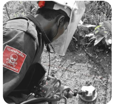
A HALO deminer uses an HSTAMIDS, a conventional metal detector which also incorporates ground-penetrating radar, to search for landmines. This kind of cutting-edge technology is one of numerous ways HALO is improving cost-effectiveness and speeding up its life saving work. The more efficient that we can make mineclearance, the more value-for-money we provide. Our work is focussed on the lands selected for clearance by beneficiaries themselves. Every extra hectare makes a difference.
