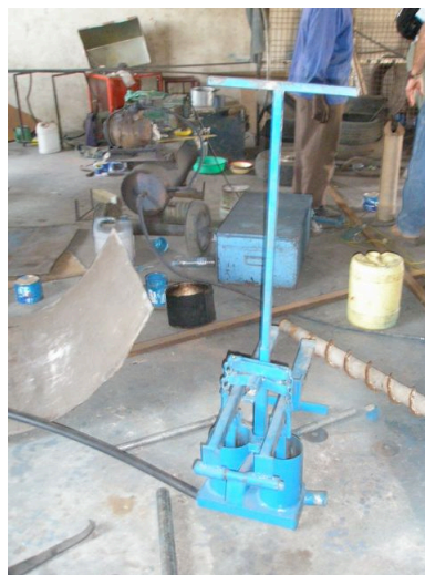
Photo: The Treadle Pump, in a workshop in Lusaka where it was being modified for use in Zambia.
