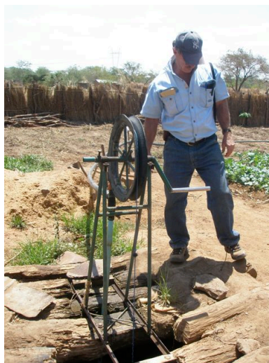
Photo: Rope and Washer pump developed by IDE and in use in Zambia.
