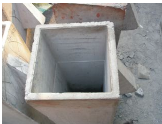
Photo: This housing for a BioSand Filter was poured near Ndola, Zambia by a local non-profit organization, SHIP. It can be made locally or bought for $65.
