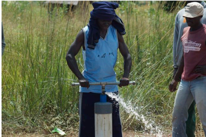
Photo: The Access2 pump working after installation on a 24-meter borehole in Samfya, Zambia
