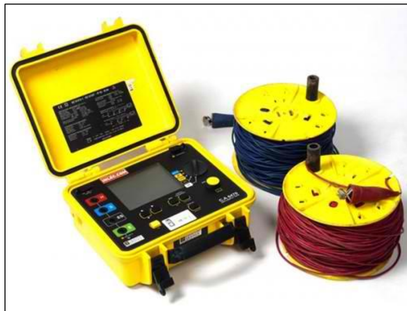
Figure 6: C.A 6472 Earth & Resistivity Tester
