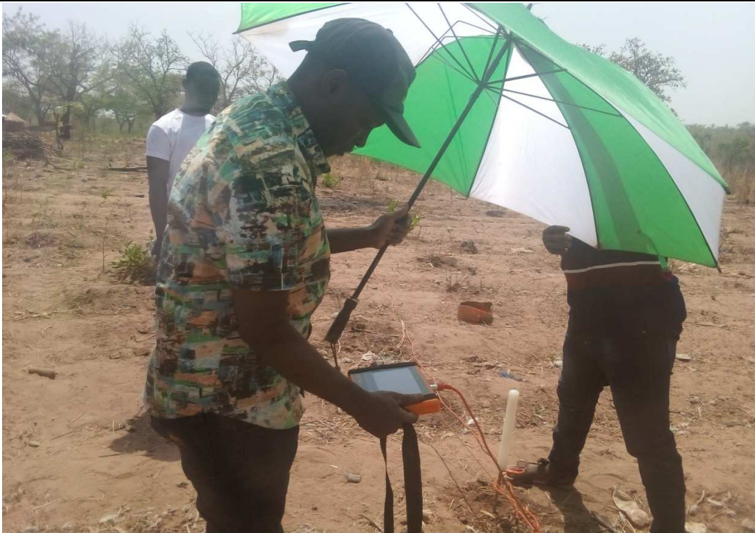
Geophysical study work for the search for groundwater before drilling
