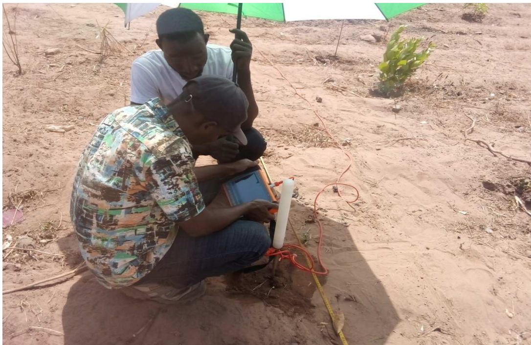
Geophysical study work for the search for groundwater before drilling
