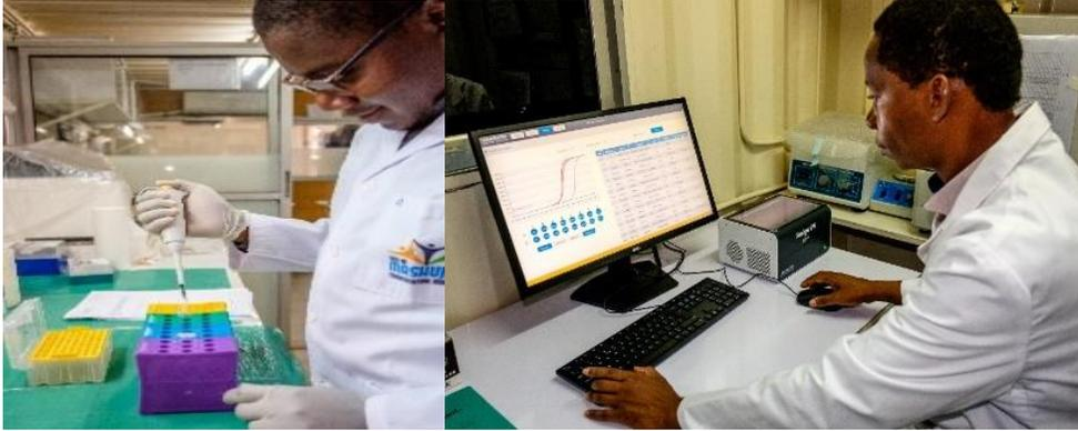
*Figure 11: Testing of waste water samples using qPCR and analyzing results*
