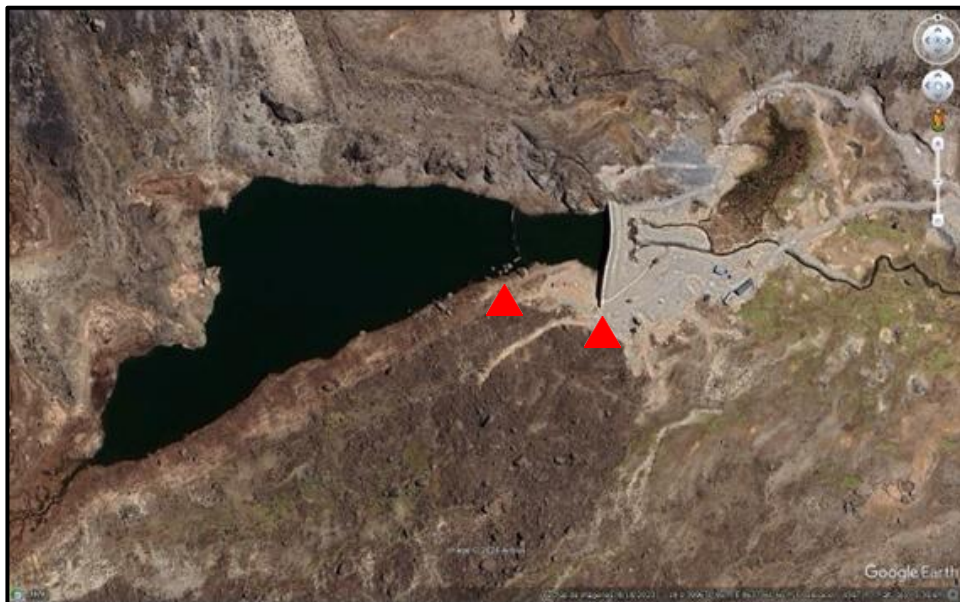
Figure 5: Satellite image showing the location and layout of Carania 3, in relation to the Mama Shiña lake. Left triangle shows the submerged old dam and the right triangle the new dam built by
