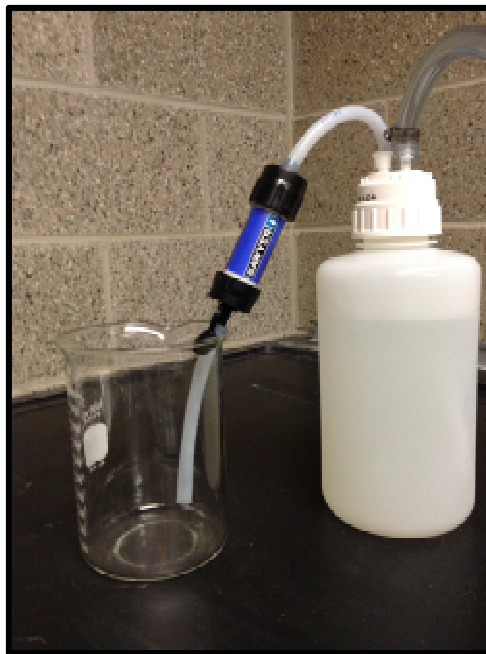
Figure 1. Pressurizing device for forcing challenge water through the Sawyer filter.
