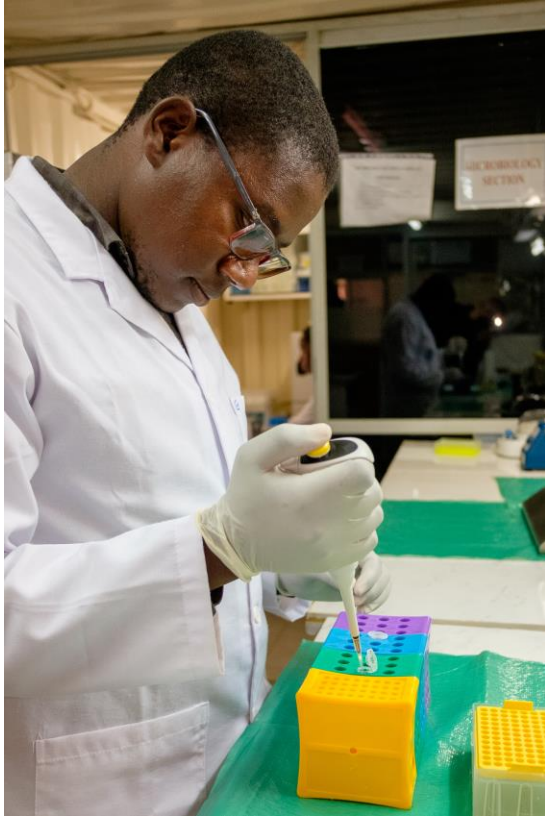
Figure 3 – Waste Water samples preparation for COVID 19 PCR testing
