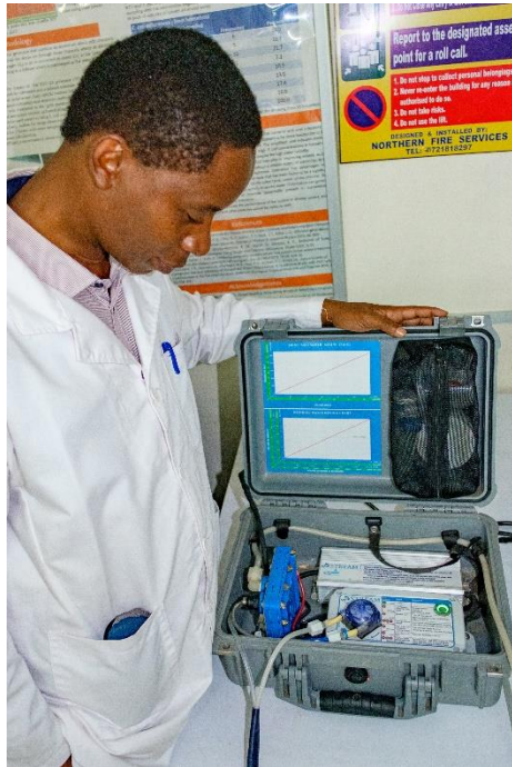
Figure 1: Lab Manager testing STREAM Chlorine Generator
