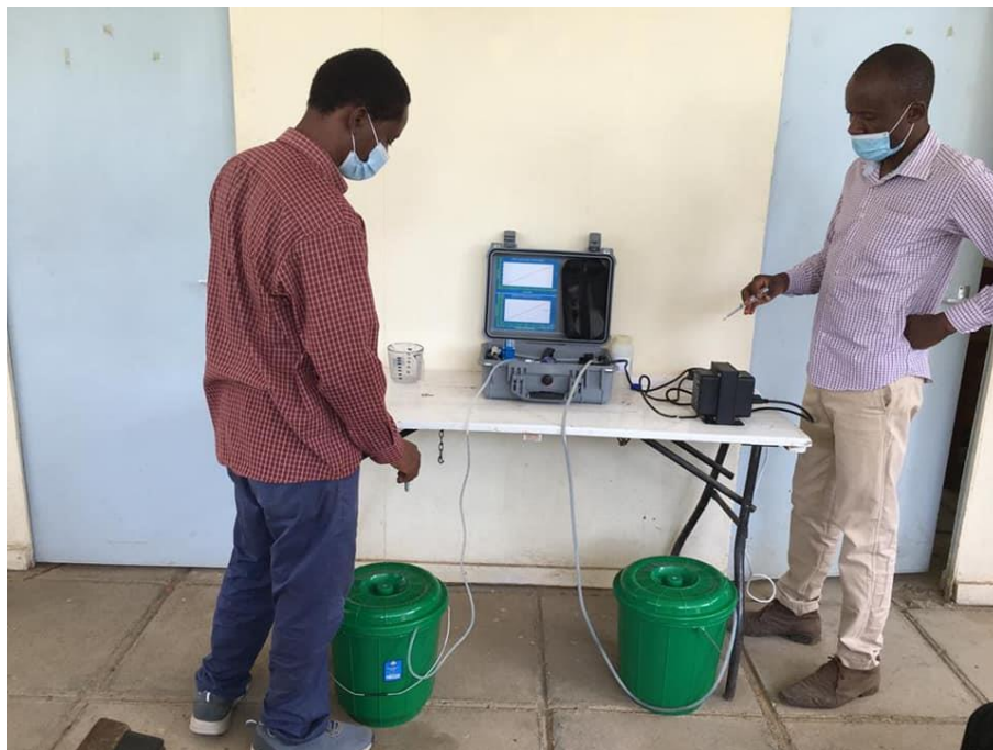
Figure 4: Production of Sodium Hypochlorite at Ahero Hospital in Kisumu County
