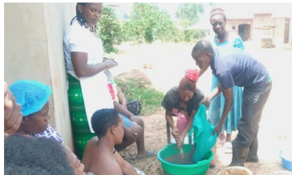
Weighing and mixing Charcoal dust, clay soil and Cassava
