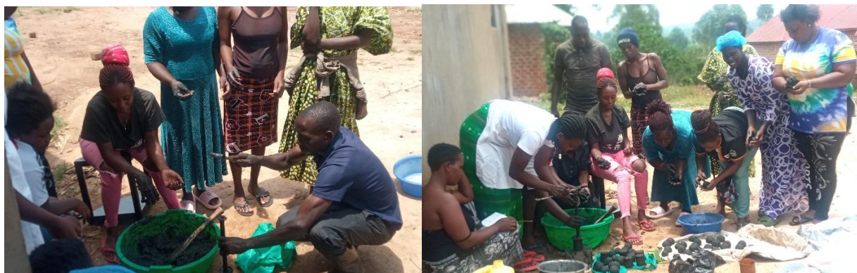
Making briquettes with a hand press and briquette balls
