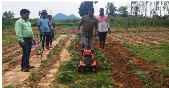
Power weeder takes 3.2 hrs per acre than 18.5 hrs
