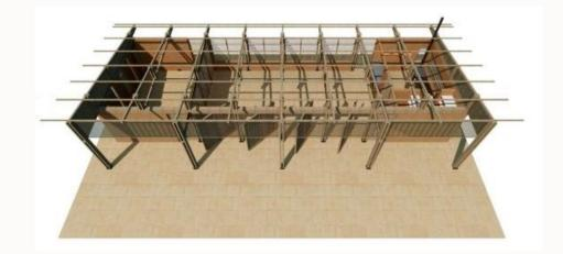
Based in traditional techniques and bioclimatic design, YANAMA will be built with wood, yorojoro (traditional cactus used for furniture and small structures), and traditional bahareque (a traditional technique mixing local sand, water and yorojoro).
