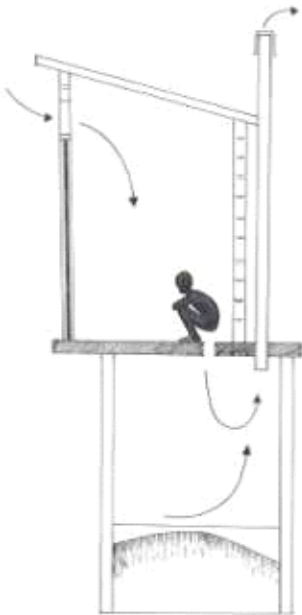
Ventilated improved pit latrine with hand-washing
