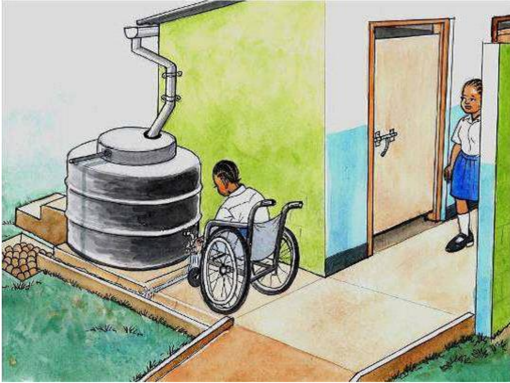
Hand-washing from a SIM tank rainwater harvesting tank next to the latrine
