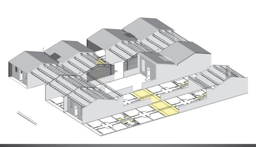
The above shows houses in various stages of development being built between shared walls. A central wayleave courtyard shown in yellow cannot be built on because this is to take common service lines of water, drainage, power etc. This means that there are two possible dwellings per 200m2 stand. The present planning in Cowdray Park is one dwelling per 200m2 stand. The owner could rent one out or sell it and live in the other.
