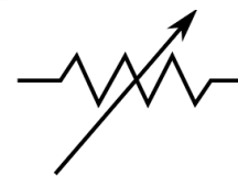
Circuit Diagram for Variable resistor ..... Symbol for Variable resistor
