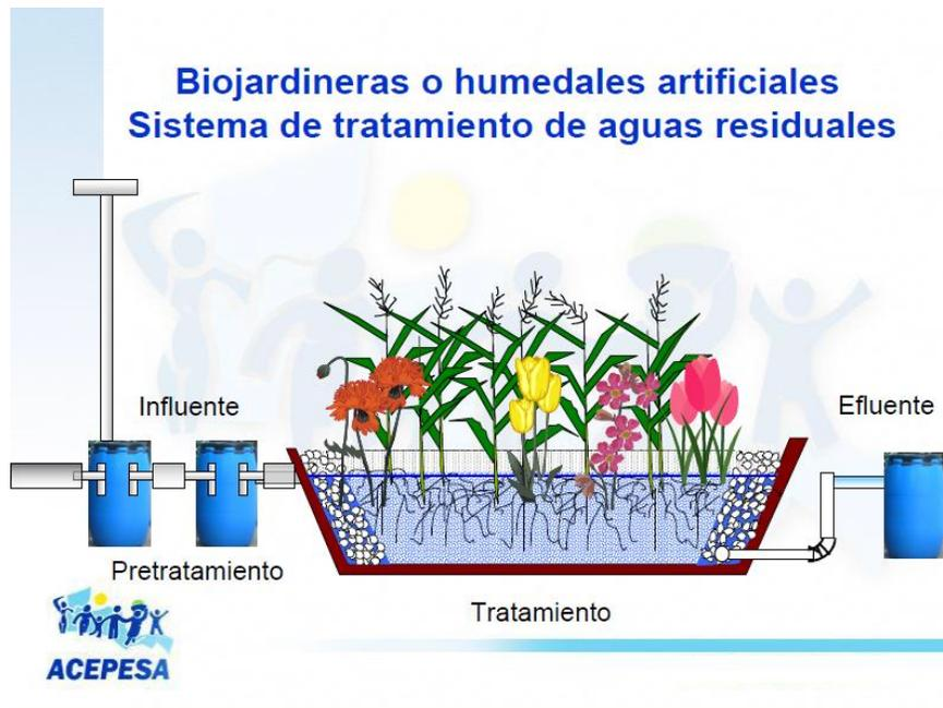
Fig. 4. Example of a biogarden system (Technological alternatives and sanitation 2015 ACEPESA.pdf)
