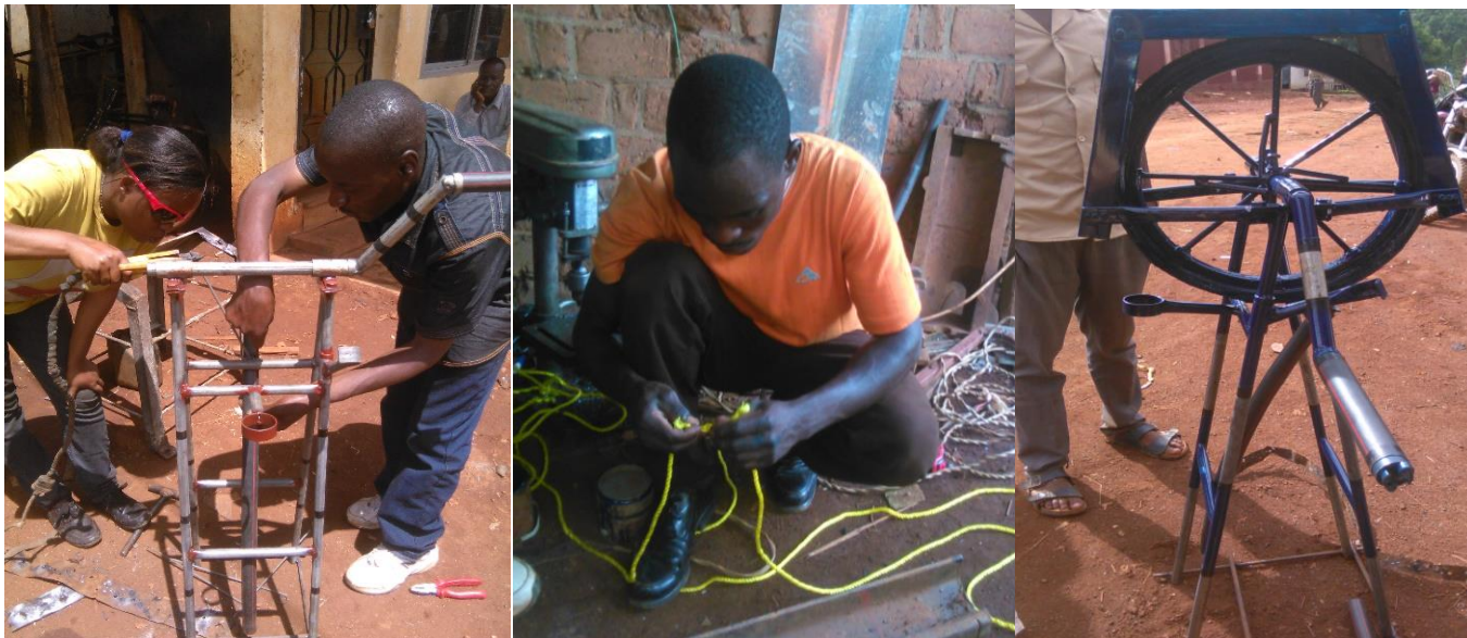
Plate 2: MVG youth building rope hand pump at Aman's Workshop in Kasulu – Tanzania.
