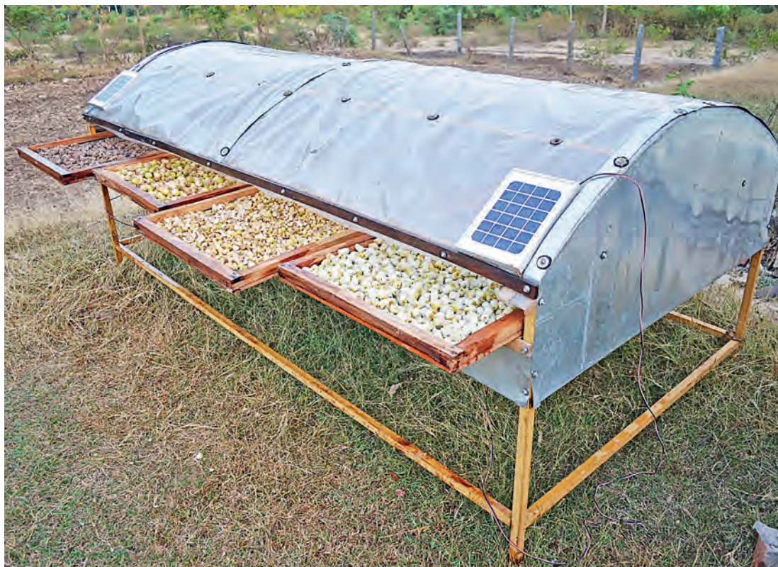
Portable solar drier for Amla
