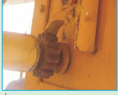
The wooden rod for changing warp side has been eliminated and replaced by a locking gear, thus no head injuries are caused.
