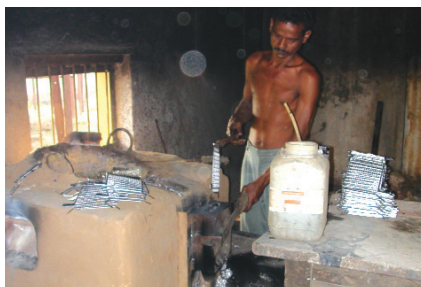
During battery manufacturing operations, lead is melted and the resulting fumes are released into the air, poisoning workers and contaminating the environment.
