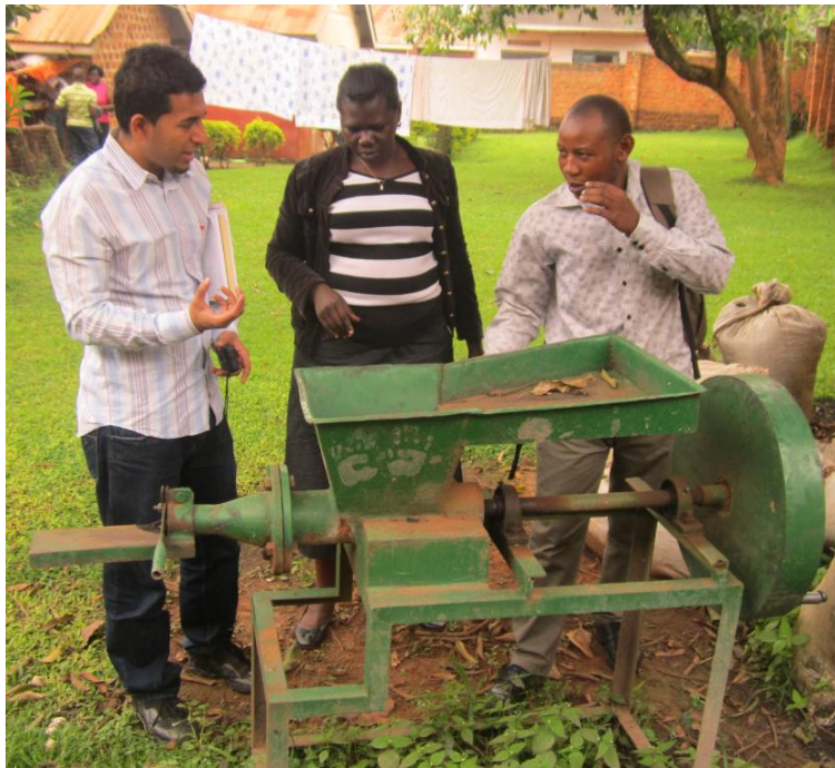
Samuel showing Ann's older design mixer and stick design machine (all manual)
