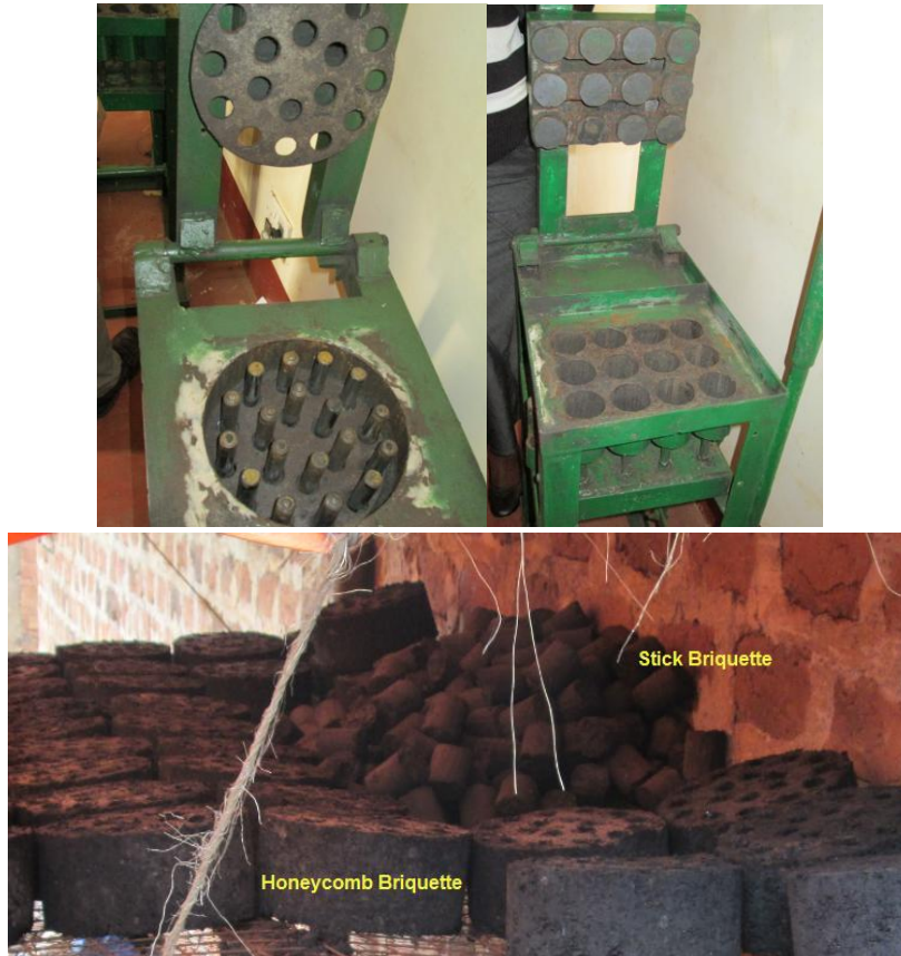
There are two design to the Briquets: Boneycomb (left) and Stick (right)
