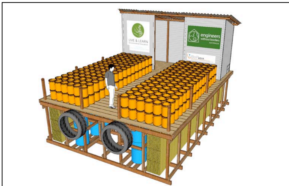
Figure 15 - Final design for the Floating Community Waste Management Station
