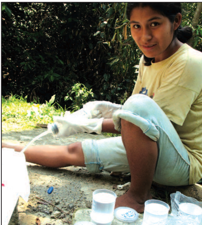
Water committee member Patti Condor, 18, conducts monthly bacteriological analysis of the water with a portable HACH lab.
