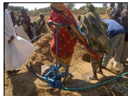
A female Agricultural Extensionist demonstrates a treadle pump for irrigation.
